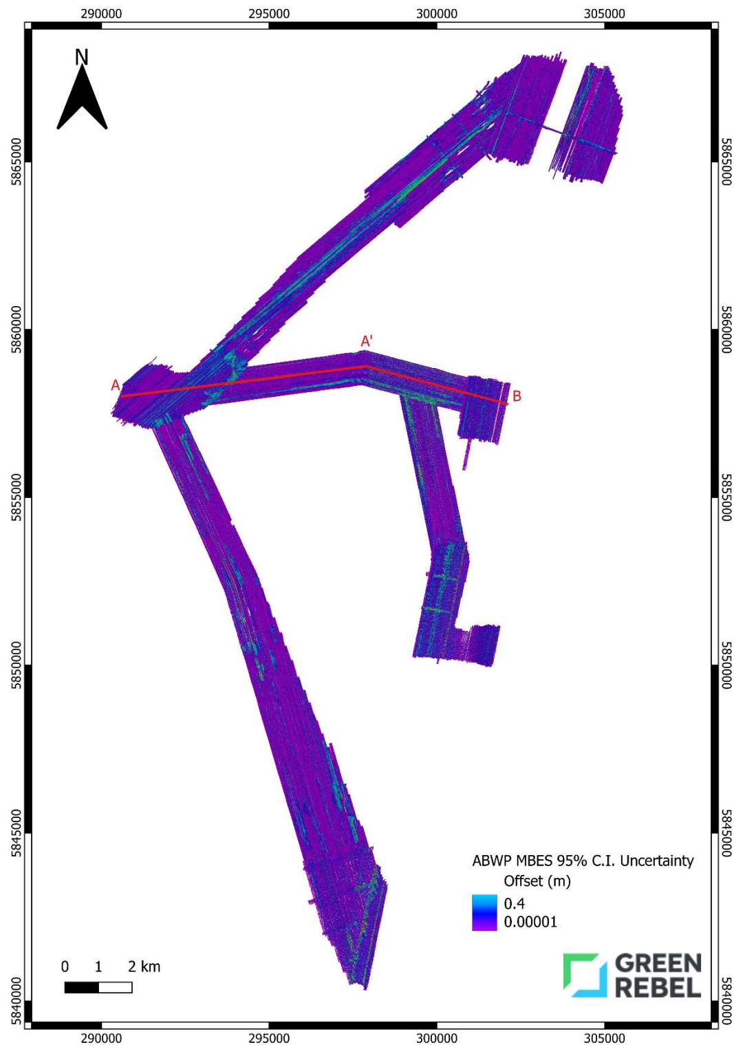
Figure 10: Multibeam bathymetric surface uncertainty (95% c.i.) and a cross profile showing the vertical alignment of adjacent survey lines (A-A'-B)
