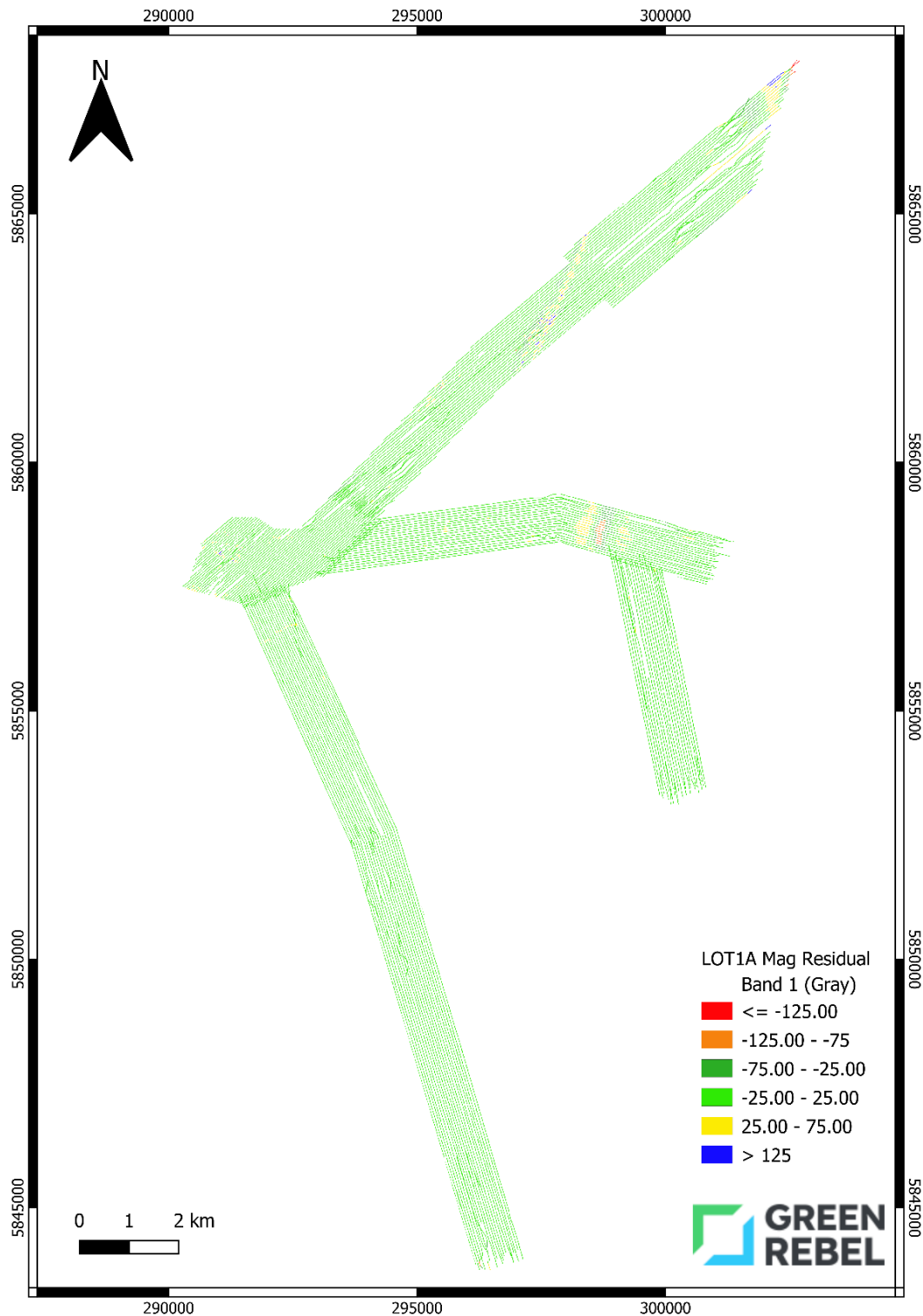
Figure 67: Residual amplitude grid across Lot 1A (pixel resolution 0.5 m)
