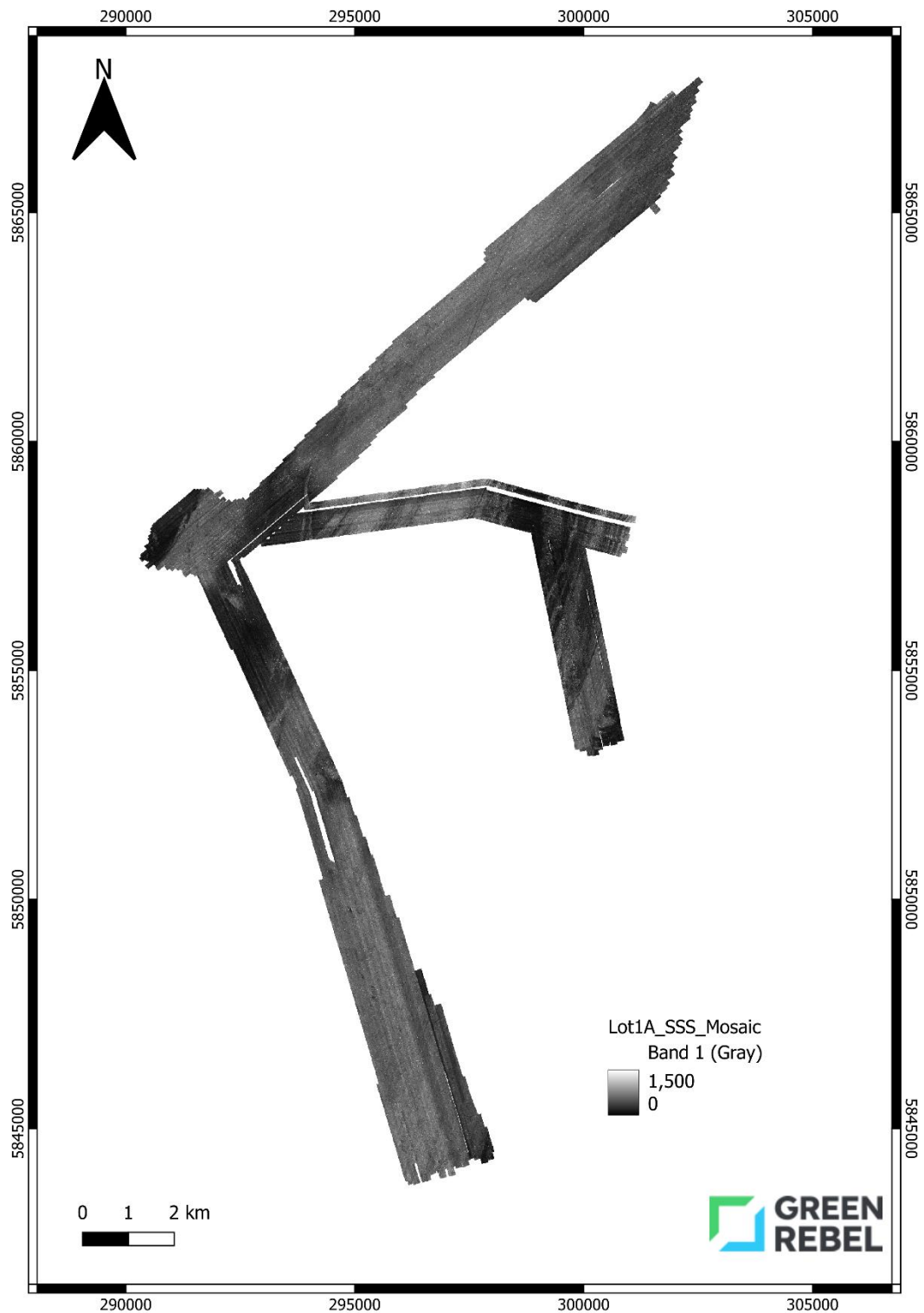
Figure 56: Low-frequency SSS mosaic from Lot 1A, presented with a pixel resolution of 0.2 m
