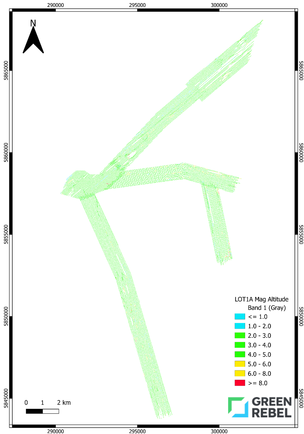
Figure 68: Altitude of magnetometer across Lot 1A gridded at 1 m pixel resolution.
