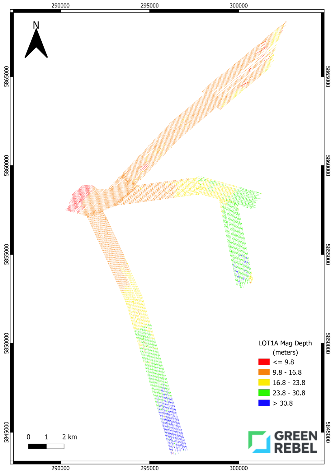
Figure 69: Depth of magnetometer gridded at 1 m pixel resolution
