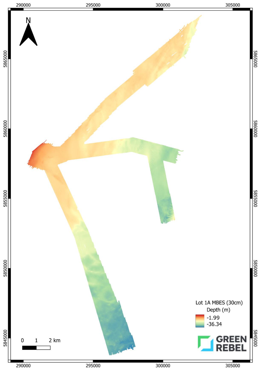
Figure 37: ABWP Lot1A bathymetric data coloured by depth (m)
