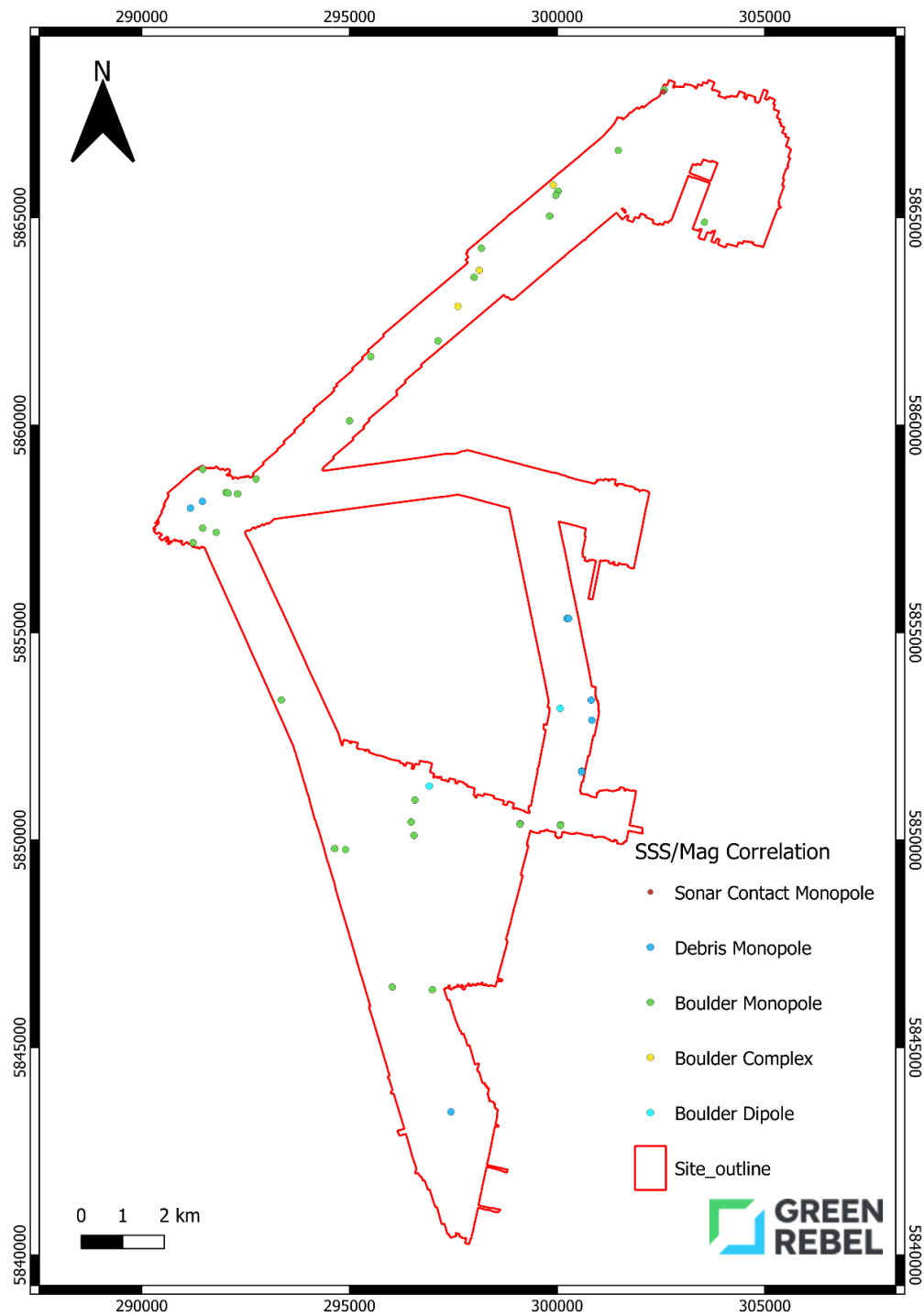
Figure 94: Identified SSS/magnetometer contacts which occurred within close proximity of each other (see Appendix 4).
